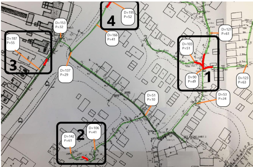
Figure 10 Example of a marked-up cable plan showing phase impedance P ( m\Omega ) and distance D (m)
