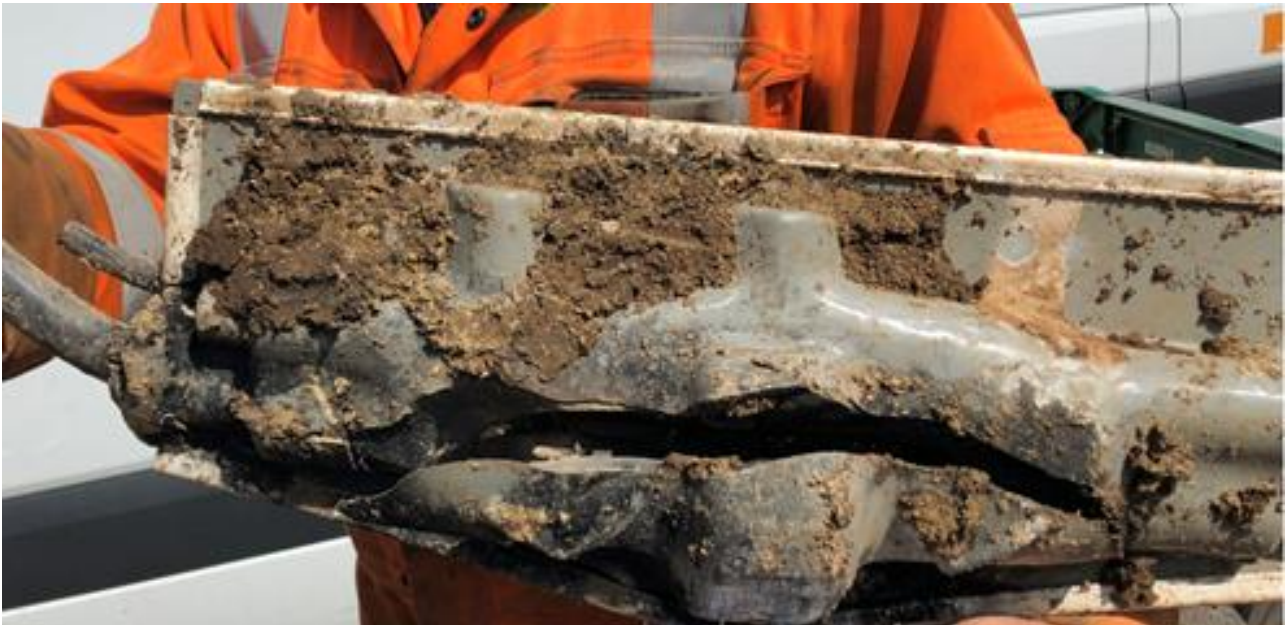
Figure 19 Recovered service joint showing signs of damage from the area of proactive fault repair
