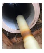
rough surface for the electromagnetic fields to focus, resulting in PD activity. Over time the amount of partial discharge activity increased, discharging between the rough outer surface of the XLPE and the oil. This correlates with the PRPD patterns recorded by the PD monitoring system and the increase in acetylene in the oil identified during DGA testing of the oil.
