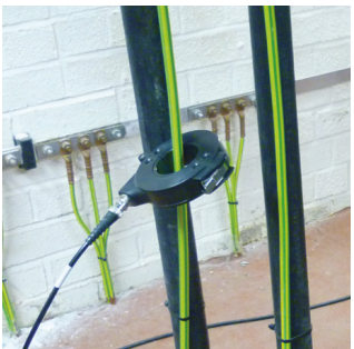
Figure 5: RFCT on earth braid of AV cable – 3 core measurement
