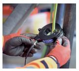
The CableData Monitor\* allows us to continuously monitor and report to you on PD activity in live cable networks. This helps to reduce the need for disruptive maintenance shutdowns by highlighting high risk areas in ample time for repairs and replacements to be
