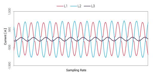
Figure 1: The current waveform of feeder 4 captured by VisNet®. The "L" labels denote the feeder phase measured.
