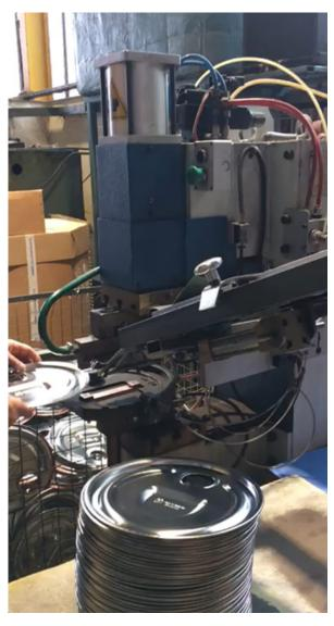
Figure 2: A spot welding machine used to weld handles on to metal lids.
