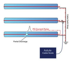
A key advantage of this approach is the significant reduction in false positives. Since permanently installed HFCT sensors allow for consistent and repeatable measurements, asset managers can differentiate between actual PD activity and external noise or transient signals. This minimises unnecessary interventions and ensures that maintenance plans are focused on genuine defects, improving network reliability and reducing operational costs.
